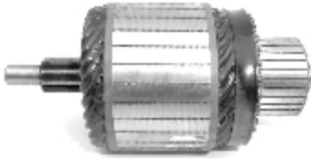
IM 3109 12 V 1.4 Kw Replacing: 230499, 23310-1S710, M106X58671, M106X58971 Servicing: 23300-1S770, 23300-1S772, M0T60081, M0T60081A, M0T60082, M0T60181, M0T60581, ... Slots:29 Teeth:9 O.D.53,7 L.113,5
