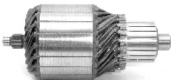
IM 604 12 V Replacing: 135815, 2110-3708200, 54290870, TGB125 Servicing: 2110-3708010, 26800, 26801, 26803, 26804, 26812, 26814, ... Slots:21 Teeth:12 O.D.54,0 L. 119,0
