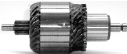
IM 3172 12 V 2.0 KW Replacing: 1004011225 Servicing: 0001125519, 0001125521 Slots:23 Teeth:11 O.D.59,0 L.143,0
