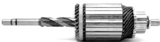
IM 53 12 V Replacing: 74351251 Servicing: MT21A, MT21B Slots: 29 O.D.73,0 L. 300,0
