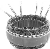
S/ 161 14 V 80 Amps Replacing: 233957, 593358 Servicing: A13VI203, A13VI236, A13VI276, A13VI278 Slots:36 O.D.127,0 I.D.96,0 H. 25,0
