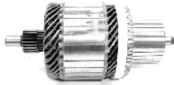
IM 3065 12 V Replacing: 10498530, 10498586, 230553 Servicing: 10465001, 10465009, 9000719, 9000735, PG200 Slots: 32 Teeth: 24 O.D. 63,0 L. 140,0
