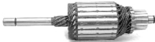
IM 601 12 V Replacing: 137530, 54292178, TGB127 Servicing: 26607, 26690, 26692, 26696, 27037, 27044, 27045, ... Slots: 21 O.D.53,6 L. 214,2
