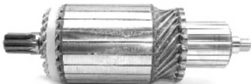
IM 3101 24 V Replacing: 0-23100-0190, 0-23100-0191, 234102 Servicing: 0-23000-1391 Slots:23 Teeth:8 O.D. 60,2 L. 188,0
