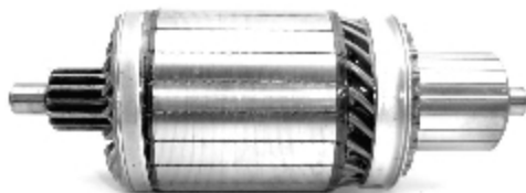
IM 3115 12 V 3.9 Kw Replacing: 233960 Servicing: 19011500, 19011505 Slots: 21 Teeth: 14 O.D. 68,0 L. 196,0
