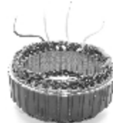
S/ 623 24 V 100 Amps Replacing: 231589, 9121334136 Servicing: 0120468143, 0120468145, 6033GB010, 6033GB023 Slots: 36 O.D.142,0 I.D.104,0 H.33,5
