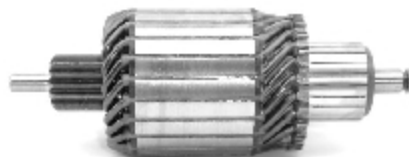
IM 2101 12 V Replacing: 068911311G, 068911311H, 077911311, 1004011022, 1004011025, 1004011031, 1004011036, ... Servicing: 0001110001, 0001110002, 0001110007, 0001110008, 0001110011, 0001110012, 0001110013, ... Slots: 23 Teeth: 15 O.D. 58,9 L. 163,0
