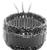
S/ 3067 12V 120 Amps Replacing: 233713, 593580 Servicing: SG12B010, SG12B011, SG12B012, SG12B015, SG12B016, SG12B018, SG12B021, ... Slots:36 O.D.135,0 I.D.106,0 H. 30,0
