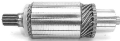
IM 3085 24 V 6.5 Kw Replacing: 132009700X0, 138964 Servicing: 03506020110, 03506020118, 03506020149, 03506020233, 03506020248, 03506020258, 03506020261, ... Slots:21 Teeth:12 O.D.65,0 L.206,5
