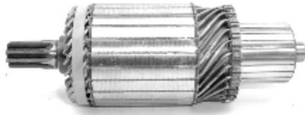
IM 3077 24 V Replacing: 132009800X0, 132009801X0 Servicing: 03505020040, 03505020069 Slots:25 Teeth:8 O.D.58,0 L.170,0
