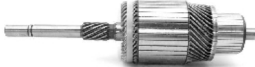
IM 953 12 V Replacing: 4172122, 74837301 Servicing: 4172119 Slots: 37 O.D. 82,6 L. 328,0
