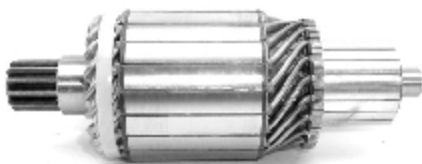
IM 3086 24 V Replacing: 132010000X0, 234108 Servicing: 03507020150, 03507020160, 03507020170, 03507020180, 03507020289, 03507020294, 03507020319, ... Slots:21 Teeth:12 O.D.75,0 L.206,0
