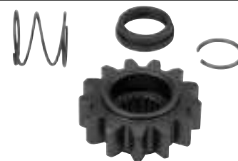
235327 Pinion Servicing: mg122433 ID 13.68, OD 39.63, Height 18.26, Splines 19, No./ teeth 13
