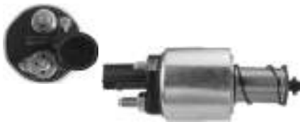
236626 Solenoid Replacing: 594743, 236626 Servicing: 191335, D6GS11, D6GS12, D6GS13, D6GS14, D7GS10, D7GS8, D7GS9, TS10E26, TS18E3 12 V, B+ M8, Kl. 50 Plug, OD 54.00, Total length 100.30, Height/ B+ 19.50, Coil bolt M8, Coil bolt 2 9.45, No./ terminals 3 Cap: HC-CARGO 236637.
