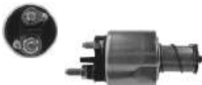
236626 Solenoid Replacing: 594743, 236626 Servicing: 191335, D6GS11, D6GS12, D6GS13, D6GS14, D7GS10, D7GS8, D7GS9, TS10E26, TS18E3 12 V, B+ M8, Kl. 50 Plug, OD 54.00, Total length 100.30, Height/ B+ 19.50, Coil bolt M8, Coil bolt 2 9.45, No./ terminals 3 Cap: HC-CARGO 236637.
