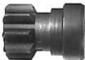
137012# Gear Wheel ID 12.00, OD 25.45, Height 36.40, No./ teeth 9
