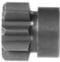
134170# Dp Gear ID 11.90, OD 25.20, Height 24.80, No./ teeth 9
