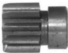
134233 Dp Gear ID 12.10, OD 25.00, Height 32.60, No./ teeth 9
