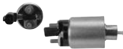
330427 Solenoid Servicing: tm000a38001 12 V, B+ M8, Kl. 50 Plug, OD 49.76, Total length 125.00, Height/ B+ 15.00, Coil bolt M8, Coil bolt 2 13.00, No./ terminals 3
