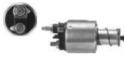
239966 Solenoid Replacing: 594459 Servicing: d7e52 12 V, B+ M8, OD 54.00, Total length 97.07, Height/ B+ 18.00, No./ terminals 2
