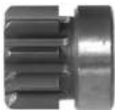
134234 Dp Gear ID 12.00, OD 25.20, Height 26.70, No./ teeth 9
