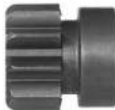
134185# Dp Gear ID 12.00, OD 27.70, Height 28.65, No./ teeth 10
