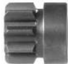
134174# Dp Gear ID 13.00, OD 25.20, Height 25.45, No./ teeth 9
