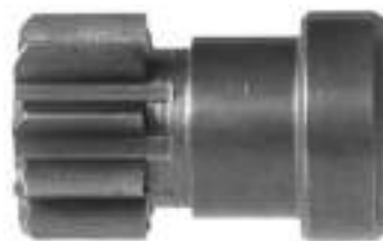
134184# Dp Gear ID 11.90, OD 28.95, Height 47.25, No./ teeth 9
