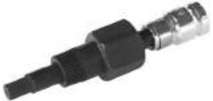
210948 Combi Tool Servicing: Audi, VW, MB, SEAT, Skoda 33 teeth combi tool for the disassembly and assembly of the free wheel pulley, XZN 10x135 mm, w/ 1/2" socket and 22 mm hexagon.
