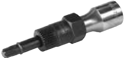
210909 Combi Tool Servicing: Valeo Alternators 33 teeth combitool for disassembly and assembly of free wheel pulley. Torx 50x110 mm, w/ 1/2" socket and 22 mm hexagon.
