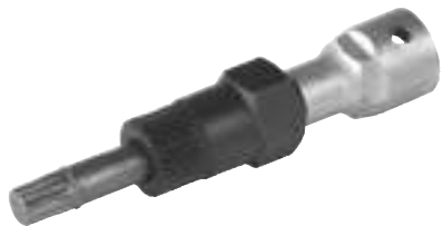
210843 Combi Tool Servicing: Bosch Alternators 33 teeth combi tool for the disassembly and assembly of the free wheel pulley. XZN 10x110 mm, w/ 1/2" socket and 22 mm hexagon.
