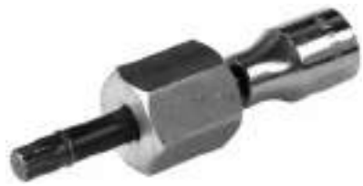
210877 Combi Tool Servicing: Bosch For removing and installing of rubber clutch pulley. XZN 10x112 mm w/ 1/2" socket and 30/28 mm hexagon.
