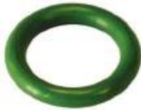
250490 O-ring Servicing: Opel, Vauxhall ID 15.47, Thickness 3.53, Material HNBR
