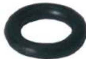
251598 O-ring Servicing: 0001416062, 0001416067, 11.139.025, 19024049, AZK5184, IM562 ID 6.00, Thickness 2.00, Material Nioprene
