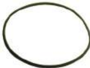
251563 O-ring ID 101.27, Thickness 2.62, Material HNBR
