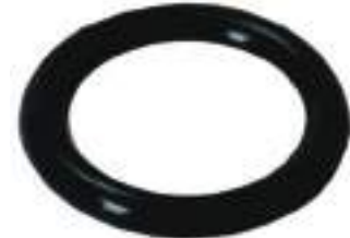
250989 O-ring Replacing: 949142-0261 Servicing: 047200-8376, 047200-9597, 147200-0262, 147200-0463, 147200-1653, 147200-1672, 147200-1982, 147200-4454, 147200-4459 ID 9.76, Thickness 1.87, Material HNBR
