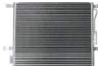
260409 Condenser Replacing: 55116931AA Servicing: Jeep Dryer w/o A: 465.00 B: 580.00 C: 28.00 mm
