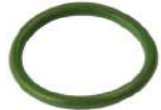
250499 O-ring ID 21.60, Thickness 2.40, Material HNBR
