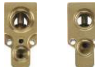
260557 Expansion Valve Replacing: 7701046080 Servicing: Nissan, Renault A: 68.15 B: 34.00 C: 49.80 mm
