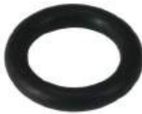
250488 O-ring Servicing: Opel, Vauxhall ID 13.87, Thickness 3.53, Material Nioprene
