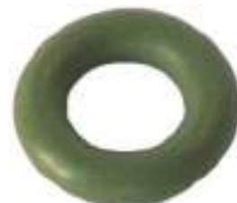
252583 O-ring ID 3.69, Thickness 1.78, Material HNBR
