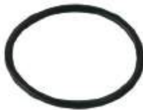
250604 O-ring ID 29.50, Thickness 2.00, Material Nioprene
