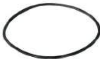
251169 O-ring ID 106.00, Thickness 3.00, Material Nioprene
