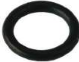
250670 O-ring ID 10.00, Thickness 2.00, Material Nioprene
