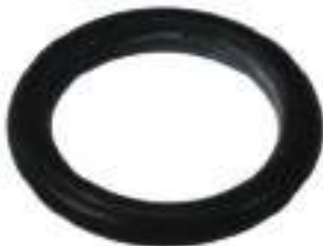
250502 O-ring Servicing: 0001416062, 0001416067, 11.139.025, 19024049, AZK5184, IM562 ID 11.91, Thickness 2.39, Material Nioprene
