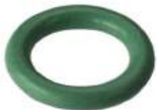
251015 O-ring ID 9.40, Thickness 2.30, Material HNBR
