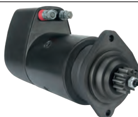
114438 Starter 24 V, 5.4 kW Replacing: 0001416032 Servicing: KHD, Liebherr, Orenstein and koppel B+ M10, B- M10, Mount. holes 3 (0), Insulated return A: 89.00 B: 47.50 mm
