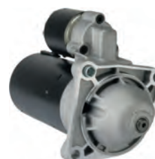
113430 Starter 12 V, 1.8 kW Replacing: AZE2111, 11.130.997 Servicing: Alfa Romeo, Fiat, Lancia, Suzuki B+ M8, Total length 226.00, Drive type Steel, Gear type GR, Mount. holes 3 (0) A: 81.50 B: 9.50 mm
