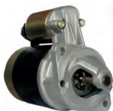
110144 Starter 12 V, 1.0 kW Replacing: 581017 Servicing: Nissan, TCM B+ M8, Total length 194.30, Drive type Steel, Gear type DD/GR, Mount. holes 2 (0) A: 82.25 B: 8.00 mm
