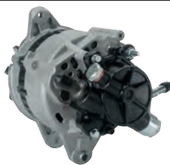
110806 Alternator 14 V, 65 Amp Replacing: HAD165500 Servicing: Mitsubishi Grooves 1, Total length 223.50, Pulley P, Fan EF A: 44.40 B: 12.80 C: 56.30 mm
