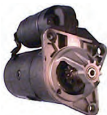
110367 Starter 12 V, 1.0 kW Manufacturer: Lucas Replacing: 6231D, 6231C, 6231B, 6231A, 6231, 6227, 6203, 6187, 6175, 6172, 6144, 6128, 532017, 532010, 532002 Servicing: Dacia, DAF, Renault, Volvo B+ M8, Total length 200.00, Drive type Steel, Gear type DD, Mount. holes 3 (0) A: 66.00 B: 10.50 mm
