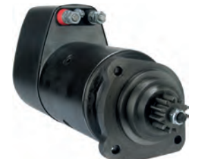
114437 Starter 24 V, 5.4 kW Replacing: 0001416031, 0001410069 Servicing: Atlas Copco, Bosch, Ford, KHD, Poclairn B+ M10, B- M10, Total length 324.00, Drive type Steel, Gear type DD, Mount. holes 3 (0), Insulated return A: 89.00 B: 47.50 mm
