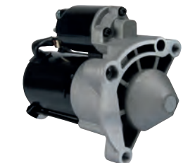
114460 Starter 12 V, 1.4 kW Replacing: 0001108400, 0001108183 Servicing: Citroen, Fiat, Hyundai, Lancia, Mitsubishi, Peugeot B+ M8, Total length 216.00, Gear type GR, Mount. holes 3 (3) B: -4.00 mm
