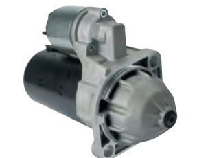
114402 Starter 12 V, 2.3 kW Replacing: 0001223022, 0001109356, 0001109355 Servicing: Mercruiser, Mercury, VM (Stabilimenti Mec) B+ M8x1.25, Total length 257.00, Drive type Steel, Gear type GR, Mount. holes 2 (0) A: 82.50 B: 16.00 mm
