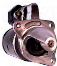
110439 Starter 12 V, 2.0 kW Replacing: 6232, 6127 Servicing: Buhner, Compair, Eicher, Massey Ferguson B+ M8, Total length 309.50, Drive type Steel, Gear type DD, Mount. holes 3 (0) A: 92.00 B: 25.00 mm
