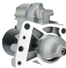
114849 Starter 12 V, 1.7 kW Replacing: 0001138006, 0001138005 Servicing: Mini B+ M8, Total length 228.00, Gear type GR, Mount. holes 4 (2) A: 60.00 B: 14.00 mm
