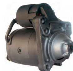
110585 Starter 12 V, 1.2 kW Replacing: 534057, 534043, 534042, 534031, 534029, 453052 Servicing: Renault, Volvo B+ M8, Total length 214.15, Drive type Steel, Gear type DD, Mount. holes 4 (4) A: 66.00 B: -2.00 mm
