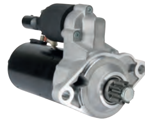
115311 Starter 12 V, 1.7 kW Replacing: 0001123037, 0001123036 Servicing: Audi, Seat, Skoda, VW B+ M8, Total length 245.00, Gear type GR, Mount. holes 2 (0) A: 76.00 B: 42.50 mm
