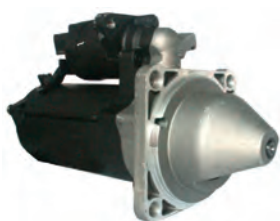
113182 Starter 12 V, 3.0 kW Replacing: AZF4155, 11.131.604 Servicing: New Holland B+ M10, Total length 320.00, Drive type Steel, Gear type GR, Mount. holes 3 (0) A: 110.00 B: 30.00 mm
