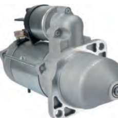
114275 Starter 12 V, 4.0 kW Replacing: 0001260004, 0001260001 Servicing: John Deere B+ M10, Total length 326.50, Drive type Steel, Gear type GR, Mount. holes 2 (0) A: 89.00 B: 48.00 mm
