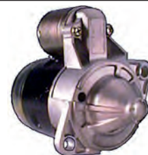
111452 Starter 12 V, 0.8 kW Replacing: S114-839, S114-780, S114-505A, S114-505 Servicing: TCM B+ M8, Total length 191.00, Drive type Steel, Gear type DD/GR, Mount. holes 2 (0) A: 82.50 B: 7.80 mm
