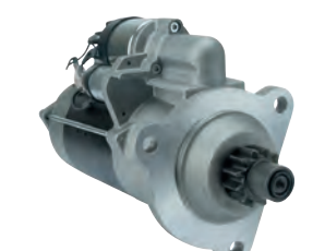
114527 Starter 24 V, 6.0 kW Replacing: 0001330004 Servicing: Volvo Penta B+ M10, B- M10, Total length 360.00, Drive type Steel, Gear type GR, Mount. holes 3 (0), Insulated return A: 92.00 B: 48.00 mm
