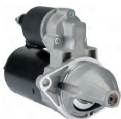
113276 Starter 12 V, 1.1 kW Replacing: AZD2126, 11.131.903 Servicing: Fiat, Mercedes-Benz, Opel, Saab, Vauxhall B+ M8, Total length 200.00, Drive type Steel, Gear type GR, Mount. holes 2 (0) A: 67.90 B: 19.00 mm
