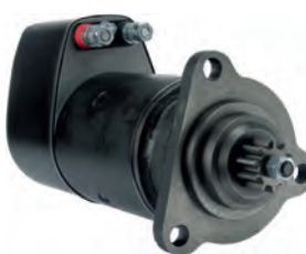
114446 Starter 24 V, 5.4 kW Replacing: 0001416046 Servicing: Iveco B+ M10, Total length 387.00, Drive type Steel, Gear type DD, Mount. holes 3 (0) A: 92.00 B: 47.50 mm
