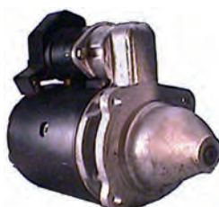
110565 Starter 12 V, 2.8 kW Replacing: 6233, 538505, 538502 Servicing: Eicher, Massey Ferguson B+ M8, Total length 313.00, Drive type Steel, Gear type DD, Mount. holes 3 (0) 4 KW: HC-CARGO 115392. A: 89.00 B: 29.50 mm
