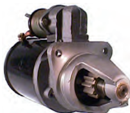
110459 Starter 12 V, 2.8 kW Replacing: 538504 Servicing: Bedford B+ M8, Total length 335.00, Drive type Steel, Gear type DD, Mount. holes 3 (0) A: 89.00 B: 47.50 mm
