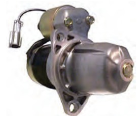
111382 Starter 12 V, 1.4 kW Replacing: S114-801D, S114-801C, S114-801B, S114-801A, S114-801 Servicing: Infiniti, Nissan B+ M8, Total length 229.85, Drive type Steel, Gear type GR, Clutch type Dry, Mount. holes 2 (0) A: 75.00 B: 56.25 mm
