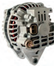
111406 Alternator 14 V, 110 Amp Replacing: HAB111100 Servicing: Dodge, Hyundai, Mitsubishi Grooves 6, Total length 170.00, Pulley SP, Fan IF A: 23.50 B: 17.25 C: 55.40 mm
