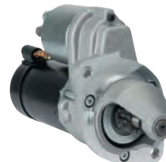
110856 Starter 12 V, 0.6 kW Replacing: 6219, 6185, 6136, 532023, 532021 Servicing: Renault B+ M8, Total length 208.50, Drive type Steel, Gear type DD/GR, Clutch type Dry, Mount. holes 2 (0) A: 66.00 B: 21.00 mm
