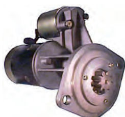
111247 Starter 24 V, 3.5 kW Replacing: S25-121A, S25-121, S24-07 Servicing: Isuzu B+ M8, Total length 243.25, Drive type Steel, Gear type GR, Mount. holes 2 (0) A: 95.00 B: 20.75 mm
