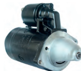
110793 Starter 12 V, 0.9 kW Replacing: 6212, 6190, 6189, 533002, 532005 Servicing: Citroen, Fiat, Peugeot B+ M8, Total length 221.00, Drive type Steel, Gear type DD, Mount. holes 2 (2) A: 66.00 B: 22.00 mm
