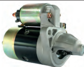
111303 Starter 12 V, 0.8 kW Replacing: S114-775A, S114-775, S114-758, S114-570C, S114-570B, S114-570A, S114-570 Servicing: Jaguar, Nissan B+ M8, Total length 185.15, Drive type Steel, Gear type DD/GR, Mount. holes 2 (1) A: 69.95 B: 11.15 mm
