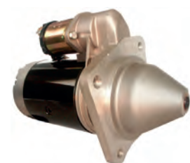
113381 Starter 12 V, 2.5 kW Replacing: AZJ3462, AZJ3195, AZJ3145, 11.139.456, 11.130.618, 11.130.510 Servicing: Farymann, Fiat, Fiat-Allis, Goldoni B+ M10, B- M8, Total length 340.00, Drive type Steel, Gear type DD, Mount. holes 3 (0) A: 109.70 B: 26.00 mm
