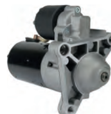
113443 Starter 12 V, 1.4 kW Replacing: AZE2534, 11.130.716 Servicing: Citroen, Fiat, Peugeot B+ M8, Total length 240.00, Drive type Steel, Gear type GR, Mount. holes 3 (3) A: 62.10 B: -5.00 mm
