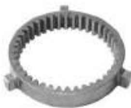
235173 Gear Wheel Servicing: 0001107072, 0001121008, 0001121009, 0001121010, 0001121011, 0001121016, 0001121017, 0001121026, 0001121027, B001120046 ID 48.50, OD 58.00, Height 10.00, No./ teeth 40
