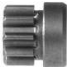
134179 Dp Gear ID 12.00, OD 26.70, Height 27.00, No./ teeth 10
