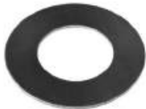
134758 DP Washer ID 29.25, OD 53.85, Thickness 1.60, Material Fiber
