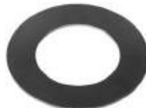
134230 DP Washer Servicing: 1006209570 ID 26.85, OD 45.25, Thickness 1.00, Material Steel
