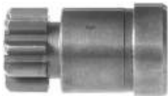
134172 Dp Gear ID 12.00, OD 25.60, Height 48.25, No./ teeth 9
