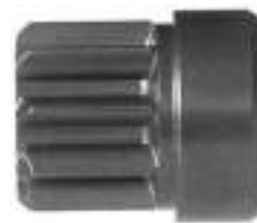
134237 Dp Gear ID 12.00, OD 25.10, Height 32.35, No./ teeth 9
