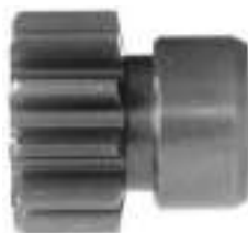
134193 Dp Gear ID 14.00, OD 40.55, Height 42.50, No./ teeth 11
