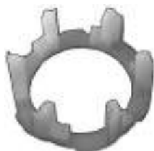
134924 Spring/roller retainer ID 33.00, OD 45.65, Thickness 17.70, Material Nylon
