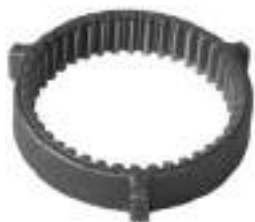
135080 Gear Wheel ID 52.23, OD 62.00, Height 13.50, No./ teeth 42
