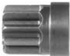
134178# Dp Gear ID 12.00, OD 25.20, Height 34.00, No./ teeth 9
