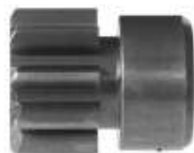
134195 Dp Gear ID 14.30, OD 34.00, Height 42.55, No./ teeth 9
