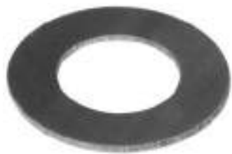
134757 DP Washer ID 24.90, OD 45.00, Thickness 1.60
