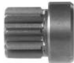
134201# Dp Gear ID 12.00, OD 25.00, Height 33.70, No./ teeth 9
