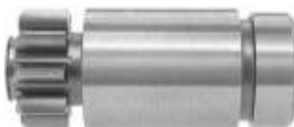
235194 Pinion Servicing: 0001124020, 0001124021, 0001125053, 0001125054, 0001125600, 0001125601 ID 11.20, OD 29.00, Height 14.50, No./ teeth 9
