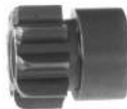
134200 Dp Gear ID 11.00, OD 25.15, Height 27.00, No./ teeth 9
