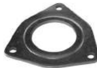
234041 Bearing Plate Servicing: A127IR, 63320277, 63320305, 63320309, 63320310, 63320315, 63320317, 63321227, 63321229, 63321231, 63321237, 63321243 ID 30.10, OD 54.50, Thickness 2.00, No./ mount. holes 3
