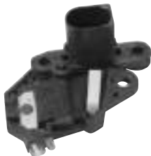
236563 Regulator Dist. mount. holes 40.00, Regulator type Electronic, Terminal type L-DFM, Battery sensor w/o, Capacitor w/, Resistor w/o, Not insulated return
