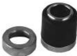
132572 Mounting Bushing Kit Servicing: 63303191, 63303780, 63304800 ID 12.30, OD 21.00, Length 29.00
