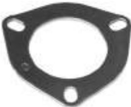
232734 Bearing Retainer Plate Replacing: 1988674, 1977674, 1911263 Servicing: 10DN, 10SI, 12SI, 15SI, 17SI, 10479809, 10479823, 10479825, 10479826, 10479827, 10479832, 10479833, 10479834, 10479838 ID 32.60, OD 56.80, Thickness 1.35, No./ mount. holes 3, Gasket w/o
