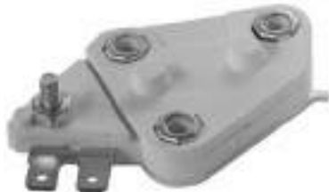
134751 Regulator Replacing: 1894460, 1116405, 1116404 Servicing: 27SI, 30SI, 10459002, 1100077, 1100078, 1100210, 1100211, 1100274, 1103132, 1105180, 1105437, 1105453, 1105454, 1105458 27.5 V setting, Dist. mount. holes 32.00, Regulator type Electronic Webbed terminals.
